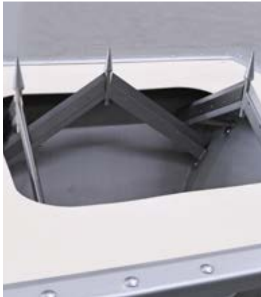
Cutting open with a U-shaped knife
