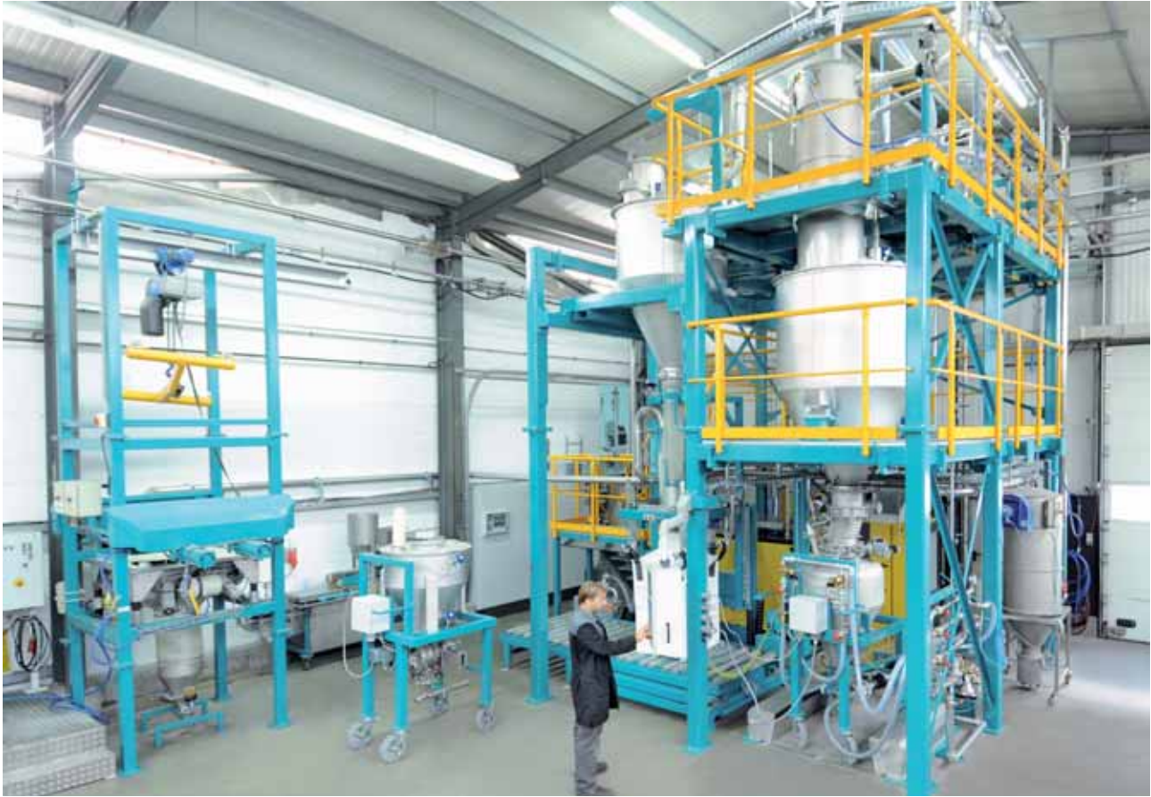
Conveyor test in the test facility pneumatic conveying
