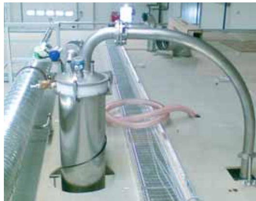
conveying of activated carbon
