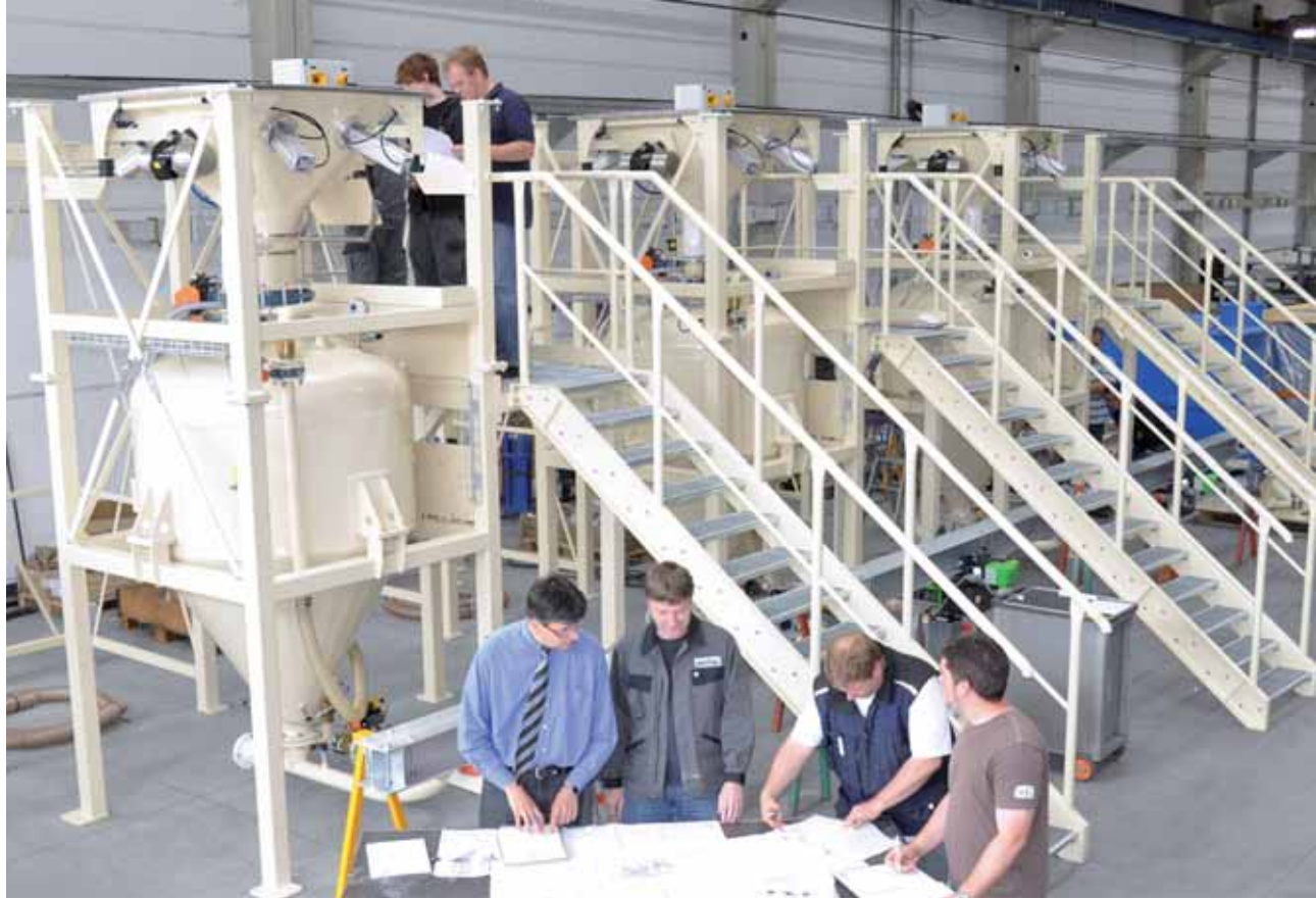
Big bag emptying station with pressure bin
