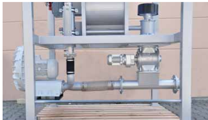
Cell wheel conveying with side channel blowers
