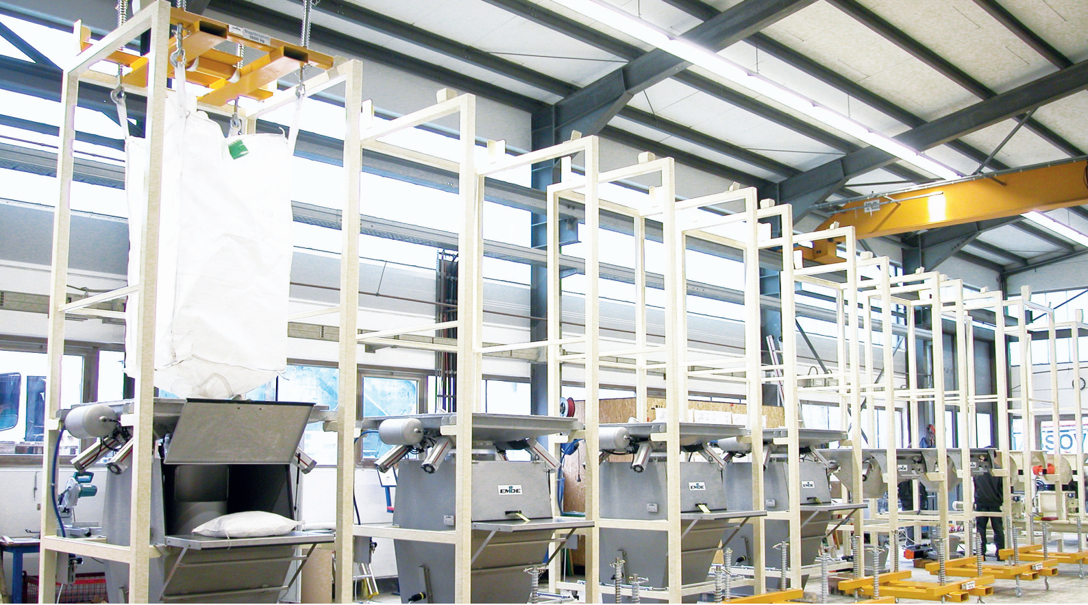
8 Combined bag/big bag emptying station in final assembly
