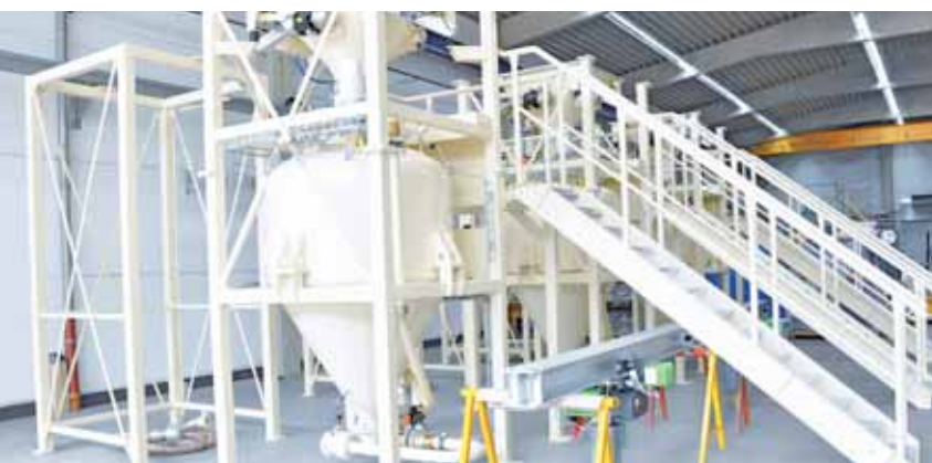
Pressure bin conveying system assembled for FAT
