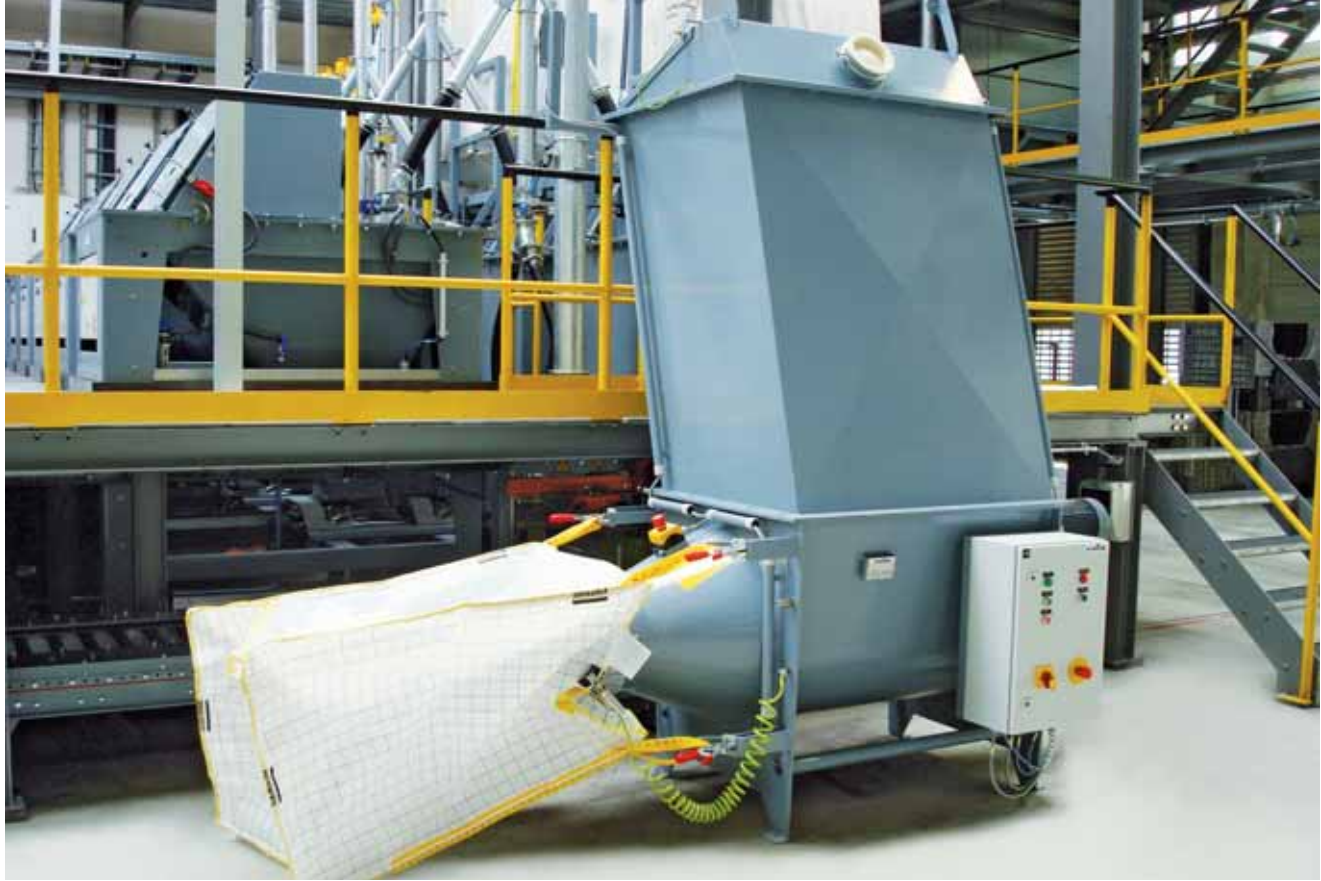
Big bag compressor with extended insertion chute
