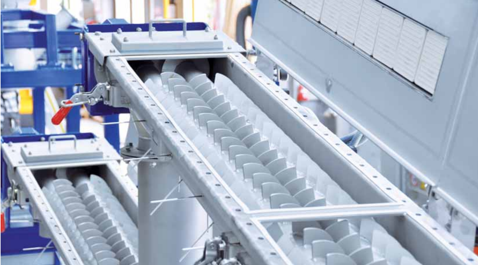
Double-paddle mixing screws with electric heating in the trough lid
