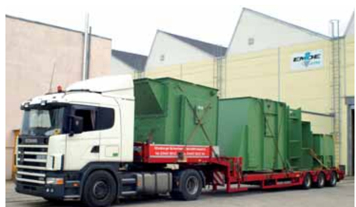
Loading bucket chain conveyor head and foot sections
