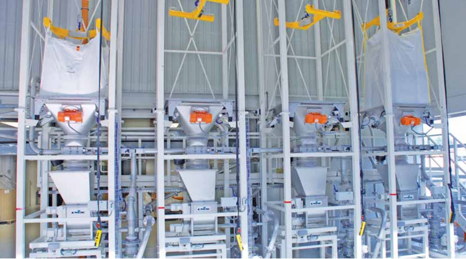
Big bag emptying and dosing equipment for plastic additives
