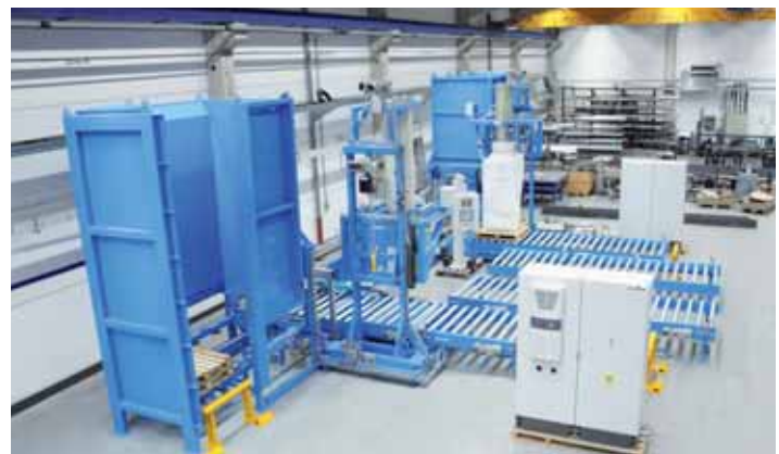
Filling equipment with pallet magazine
