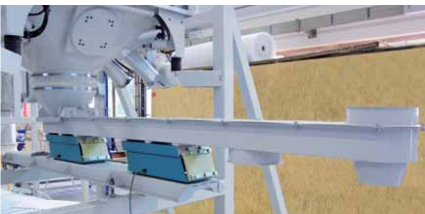
Product dosing from big bag discharge with magnetic oscillating conveyor
