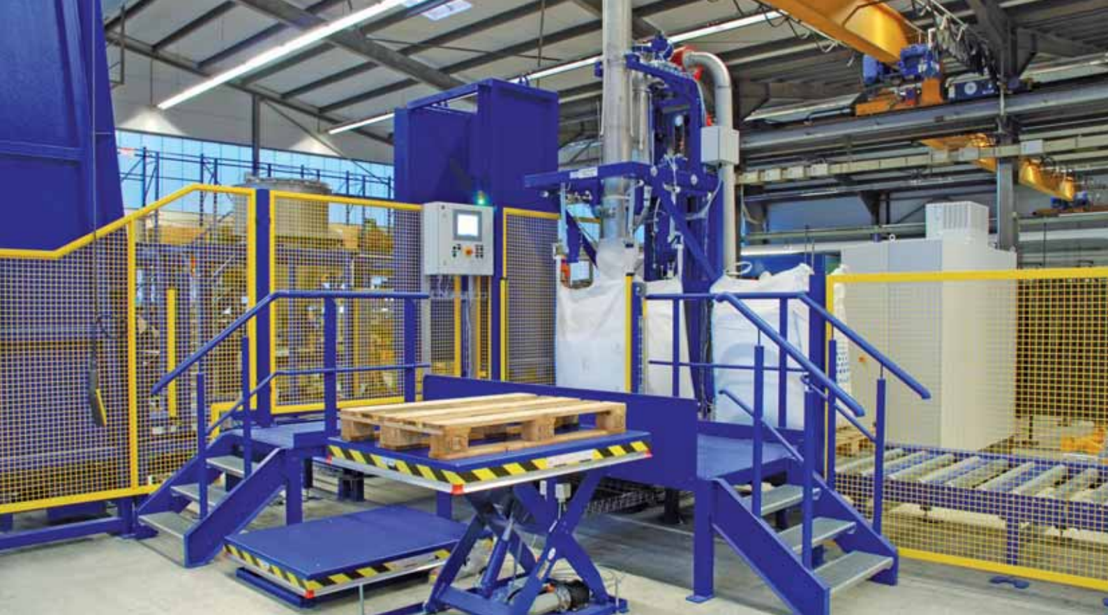
Big bag filling plant with pallet magazine and conveying technology for pallets
