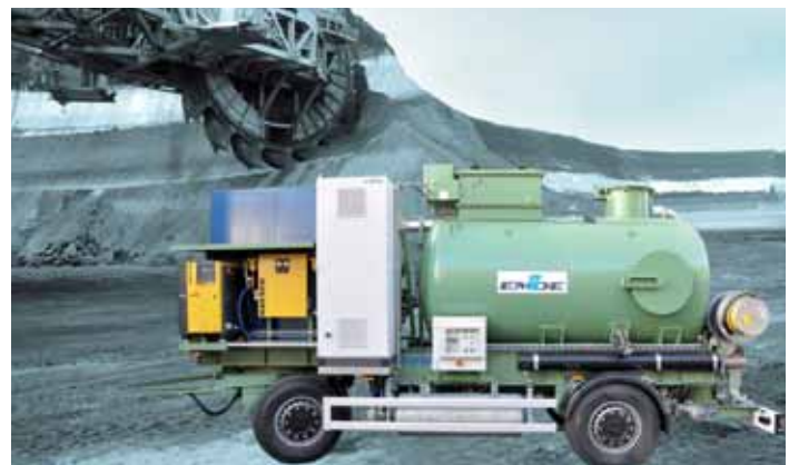
Mobile vacuum cleaning system for ash
