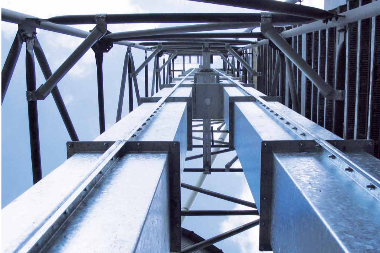
Bucket elevator for transporting grain
