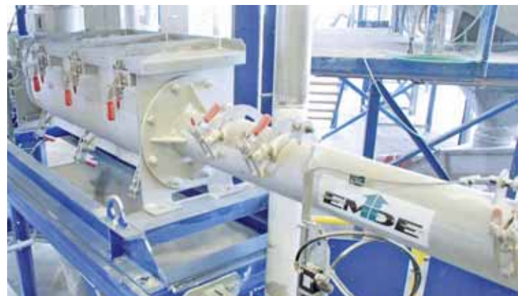
Throughput mixer for adding iodine to salt
