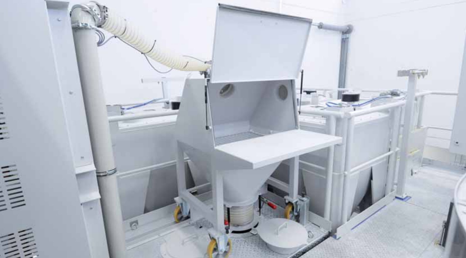
Sack chute with discharge docking
