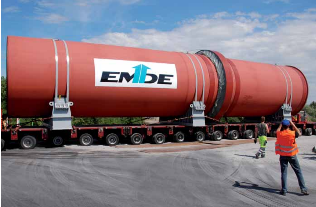
Transporting a rotary furnace segment
