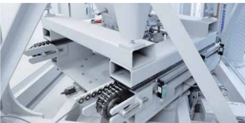
Shuttle transport with chain conveyor and rotary table
