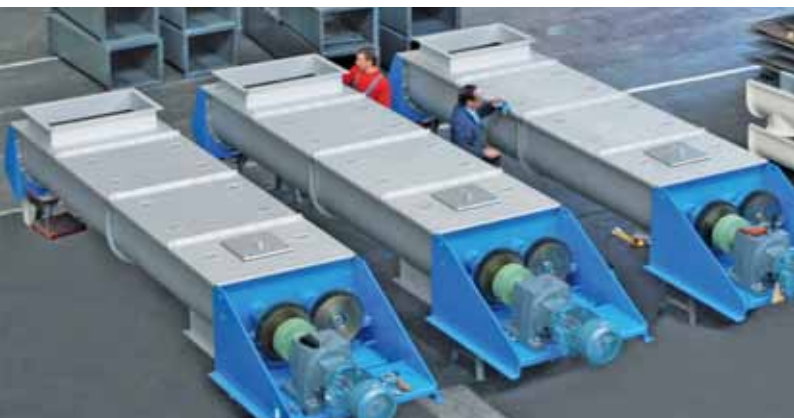
Final assembly of dual screw conveyors
