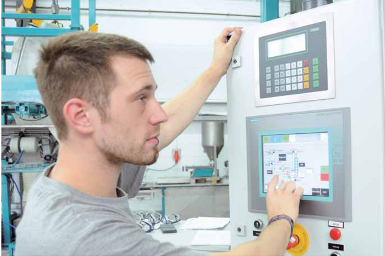
Control unit with operating panel and scale evaluator unit
