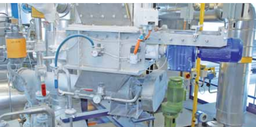
Twin-shaft lump breaker in the plastics industry
