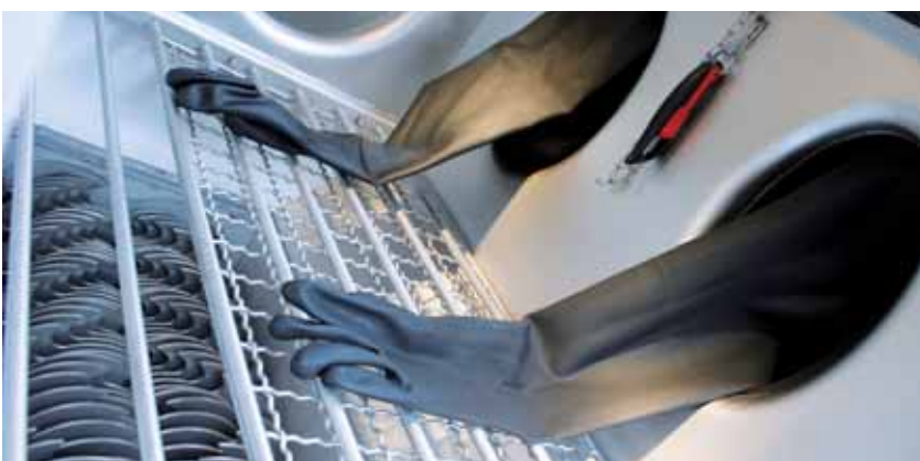
Interior view of the sack emptying cabin with downstream lump breaker
