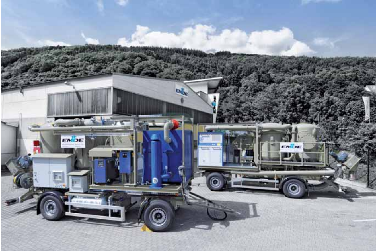
Mobile vacuum units for flexible deployment on pipeline networks
