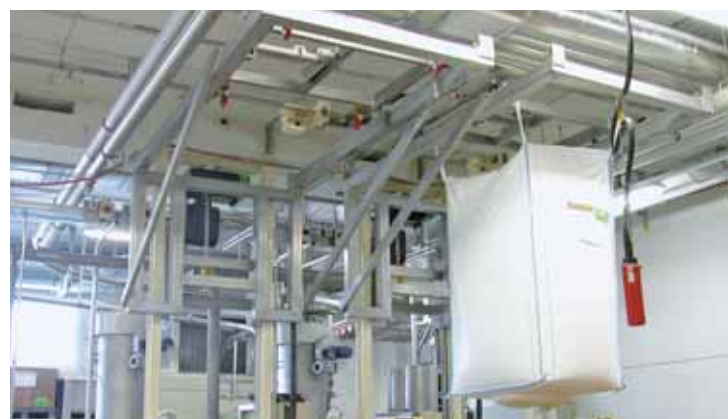
Big bag emptying with building height-reduced lifting column
