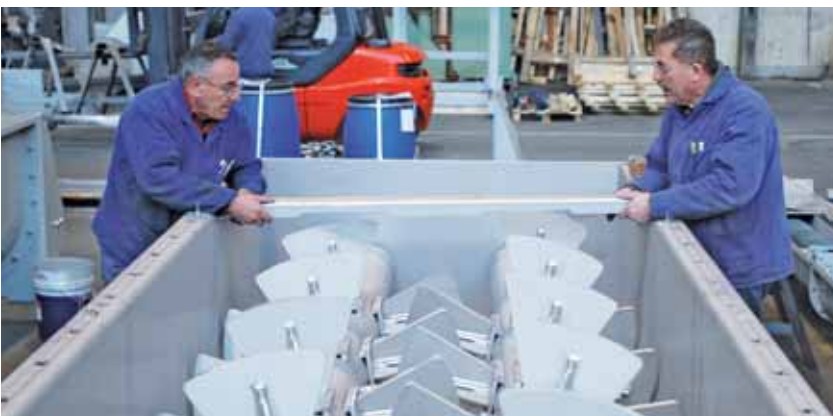
Dual paddle mixing screw in final assembly
